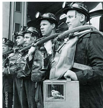
The origins of portable gas detection technology are found in the mining industry. Before the availability of sensors, canaries acted as a warning system for alerting miners to hazardous substances in the mine.
