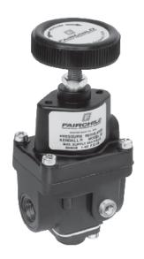
The Model 30 is designed for applications that require high capacity and accurate process control. A supply valve which is balanced by utilizing a rolling diaphragm, insures a constant output pressure even during wide supply pressure variations. Stability of regulated pressure is maintained under varying flow conditions through the use of an aspirator tube which adjusts the supply valve in accordance with the flow velocity.
