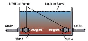
Heating Liquid In-Tank with Model CTE Liquid or Slurry
