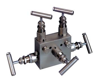
The DPM is a five-valve power/vent pattern manifold for rack or pipe-stand mounting to a differential pressure transmitter that enables instrument operation, isolation, zeroing, calibration and venting in a single unit suitable for liquid, steam or vapor service.
