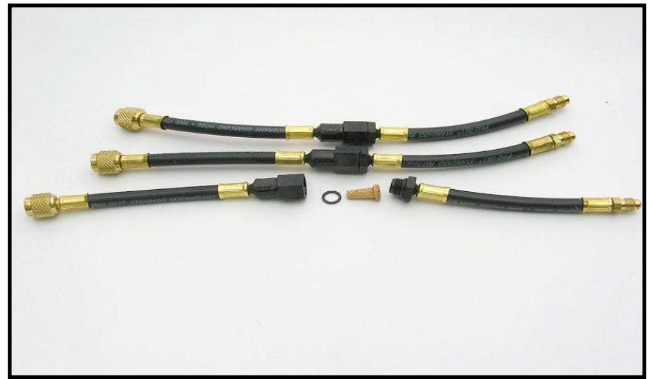
Part No. 109445 Filter Assembly Adapter Kit Set of 3 -12" hoses. For Test Kit Hoses that do not have filters. 1/4" Quick Coupler x 1/4" Flare Connection. Field serviceable filter housing and filters included.
