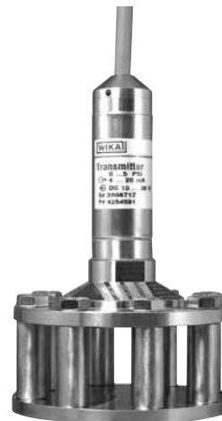
Optional WIKAI LevelGuard Anti-clog attachment for submersible level transmitters. For use in lift stations, wet wells and other difficult level applications. For more information request bulletin LG-1.
